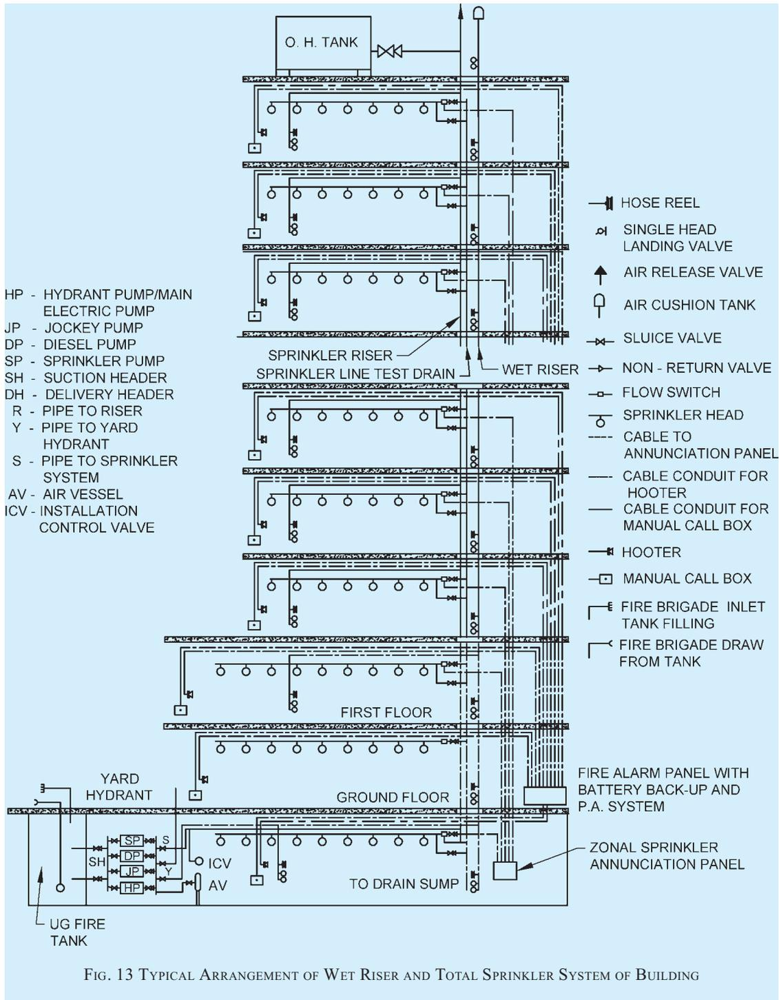
FIG. 13 TYPICAL ARRANGEMENT OF WET RISER AND TOTAL SPRINKLER SYSTEM OF BUILDING
