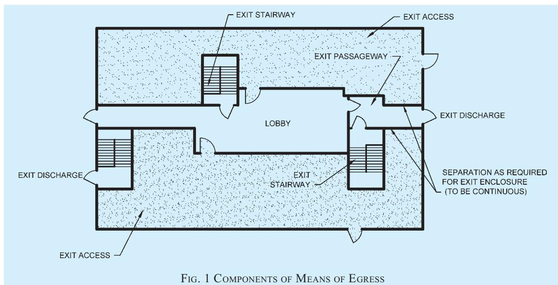
FIG. 1 COMPONENTS OF MEANS OF EGRESS
