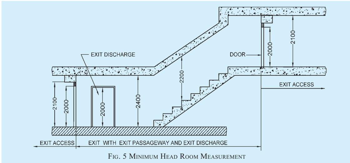
FIG. 5 MINIMUM HEAD ROOM MEASUREMENT
