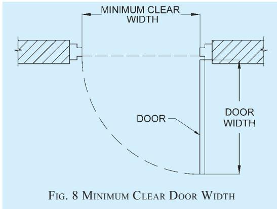
FIG. 8 MINIMUM CLEAR DOOR WIDTH
