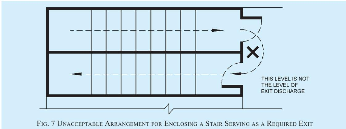
FIG. 7 UNACCEPTABLE ARRANGEMENT FOR ENCLOSING A STAIR SERVING AS A REQUIRED EXIT
