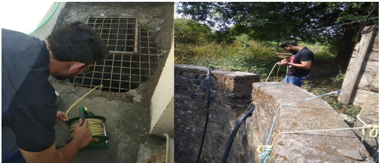
Figure 6.10: Measurement of groundwater level using automatic water level indicators
